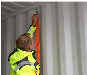
1. Attach the safety hooks to the top and bottom of the container eyelet.
